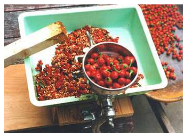
Figures 2 and 3: Illustration of a Corona grain mill, and photo of a Corona mill being used to extract the seed of a small-fruited hot pepper ('Amazzo'). The wooded "push rod" is used to force the uncut fruit into the throat of the hopper and between the threads of the auger. Small hot peppers do not need to be cored or sliced. The mash is caught in a large tray and later transferred to a bucket for fermentation. When working with small-fruited varieties, quite a bit of seed (ounces to pounds) can be extracted this way.
