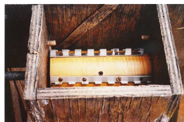
Figure 9. Throat of an apple grinder made from a kit. Photo courtesy of Merlyn Niedens.
